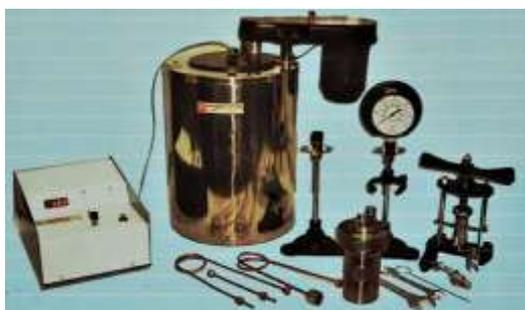
Figure: 4.Digital Bomb calorimeter [8]
