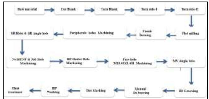
Fig. 2: Process sequence of 3 Axis Machining center
