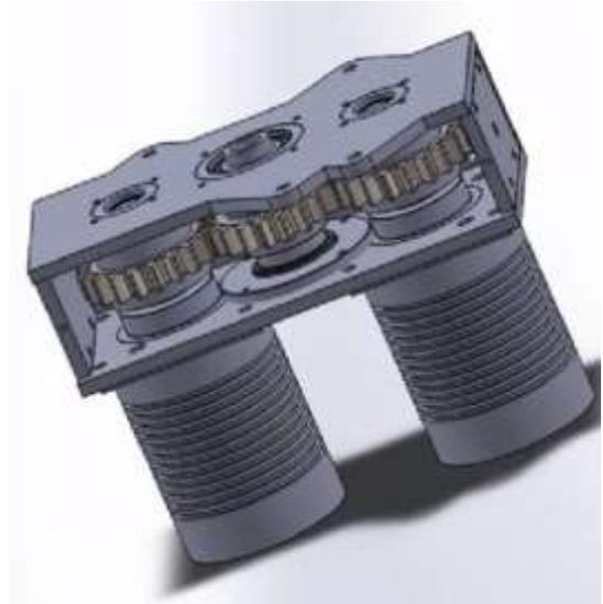
Fig. 2: Model of Multi-motor coupling
