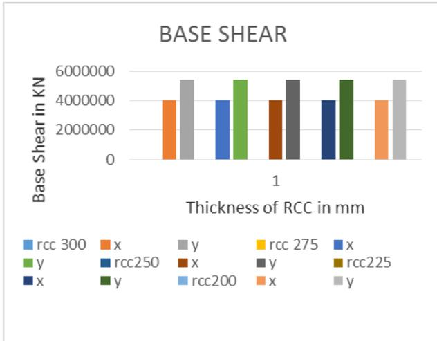
Fig 3: Base shear of RCC shear wall
