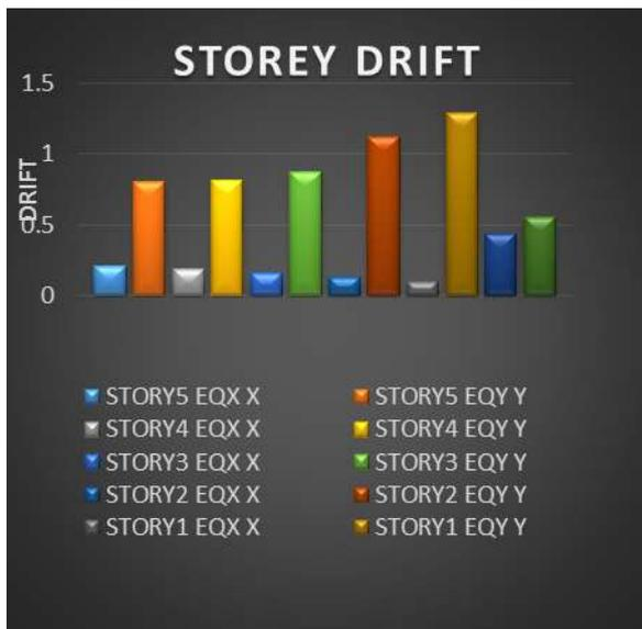
Fig 10: Storey drift of 300 mm thick RCC shear wall
