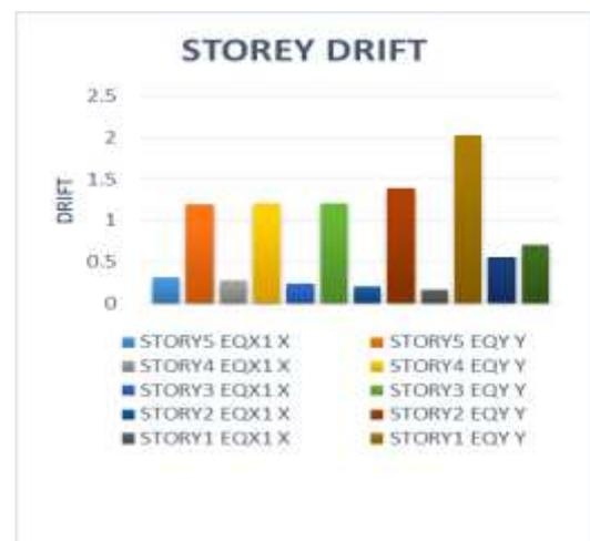
Fig 12: Storey drift of 26 mm thick Steel Plate shear wall
