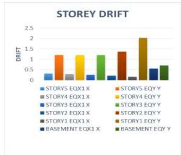
Fig 11: Storey drift of 24 mm thick Steel Plate shear wall
