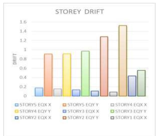
Fig 19: Storey drift of 30 mm thick composite shear wall
