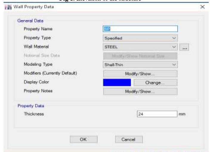
Fig 2: Assigning thin-Shell elements for steel plate in ETAB version 2016
