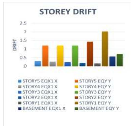
Fig 13: Storey drift of 28 mm thick Steel Plate shear wall
