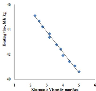
Fig. 7: Influence of viscosity on heating value of blends
