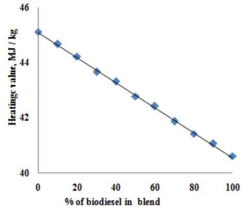
Fig. 4: Influence volume fraction of biodiesel on heating value of blends
