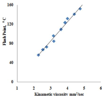
Fig. 6: Influence of viscosity on flash point of blends
