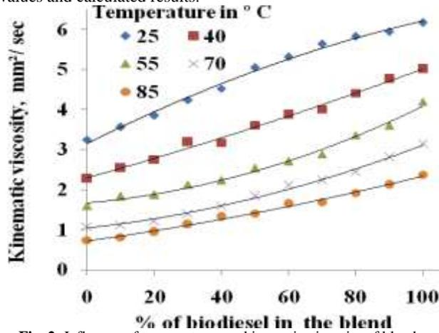
Fig. 2: Influence of temperatures on kinematic viscosity of blends.
