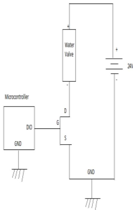
Fig. 5: Circuit Diagram of the System
