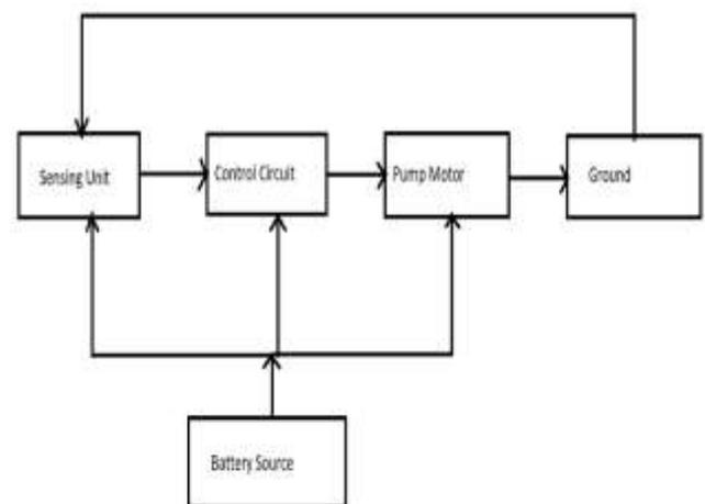
Fig. 1: The system block diagram of automatic irrigation system
