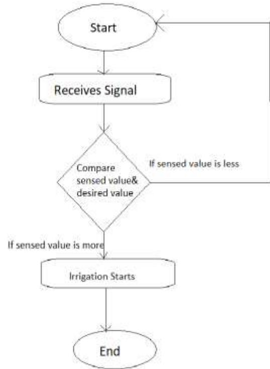
Fig. 3: Flowchart relates soil moisture sensor and the Arduino controller.
