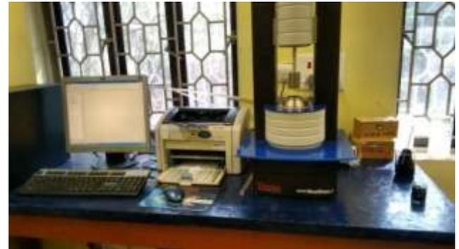
Fig. 2.2: Rheology test of CWS with HAAKE RHEO STRESS 1
