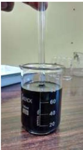
**Fig. 2.3:** Stability test with rod penetration
