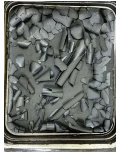
**Fig. 2.4:** Particles below 37  $\mu$ m**3.3. Maximum Static Settled Concentration ( $C_w$  Max %)**
