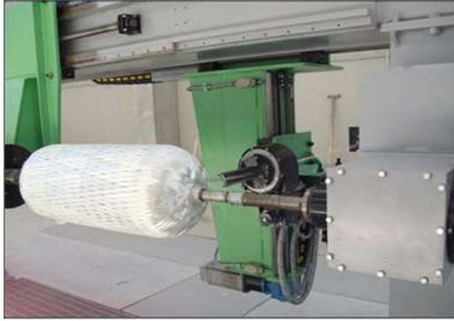
Fig. 2 Filament winding technique
