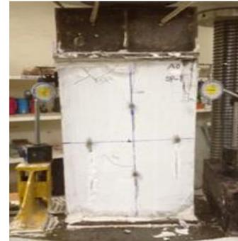
Fig. 10. Axial load test setup
