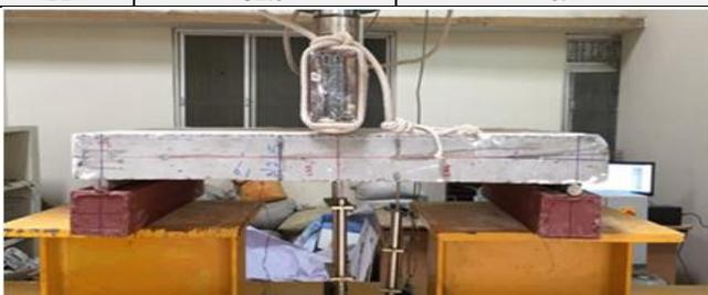
Fig. 3. Flexural strength test setup
