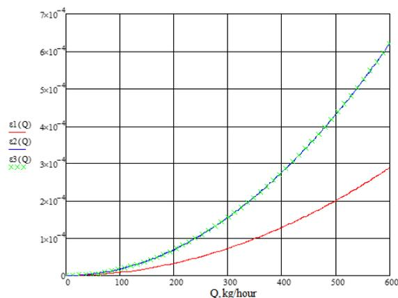
**Fig 6:** The dependence plot of strain gauge relative strain absolute value on the mass flow rate of air
