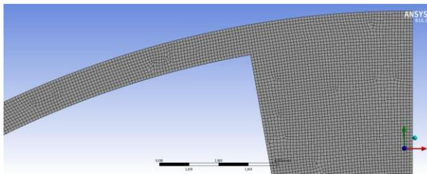
**Fig 3:** Transducer final element mesh
