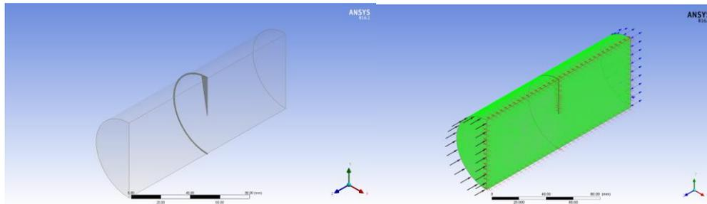
**Fig 1:** Assembly geometry adjusted in Design Modeler **Fig 2:** The setting of properties for Air domain
