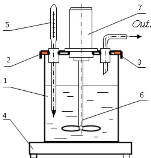
**Fig. 3:** Laboratory setting for adsorbent preparation: 1 - glass; 2 - cover; 3 - sealant; 4 - heater; 5 - thermometer; 6 - mixer; 7 - electric motor of the mixer.
