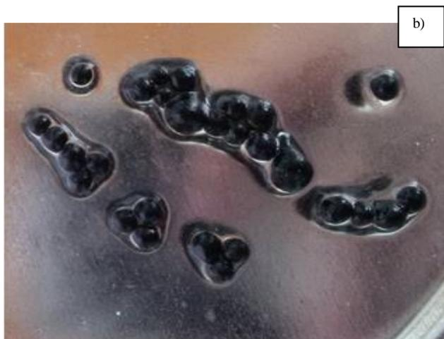
**Fig. 5:** Characteristics of the granulation process: a) - chitosan granules; b) - composite granules of chitosan with modified sunflower husk
