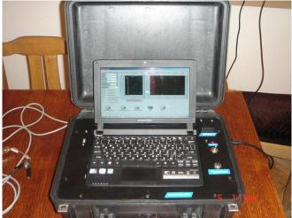
Fig. 3: Device for assessing the frame insulation condition in electrical machines of locomotives.
