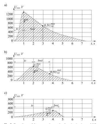
**Fig. 2:** Dependence of the return voltage value from its rise time and fall time: a) new insulation, TM mileage  $L_0$ ; b) after a certain period of operation  $L_1$ ; c) worn insulation, period of operation  $L^*$ .
