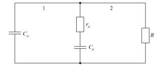
**Fig. 1:** Equivalent scheme used to consider the absorption process taking into account leakage currents.
