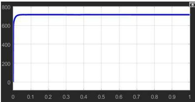
**Fig.6:** Output Voltage of Battery fed Superlift Luo Converter
