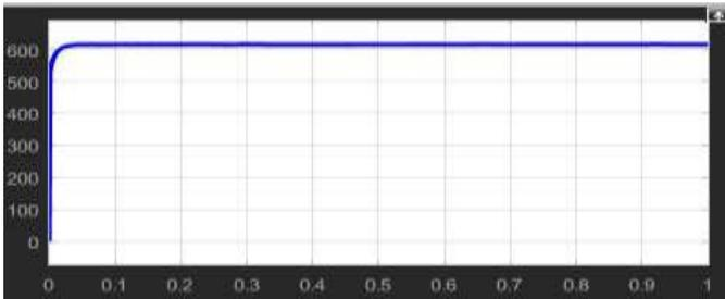
**Fig.5:** Output Voltage of Constant DC Source fed Superlift Luo Converter
