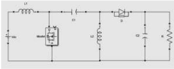
Fig.1: Equivalent Circuit diagram of Zeta Converter
