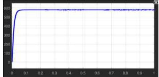
Fig.2: Output Voltage of Constant DC Source fed Zeta Converter
