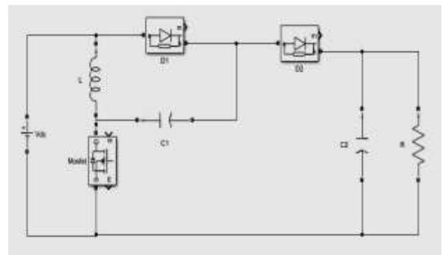
Fig.4: Equivalent Circuit diagram of Superlift Luo Converter
