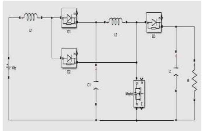
**Fig.7:** Equivalent Circuit diagram of Cascaded Boost Converter
