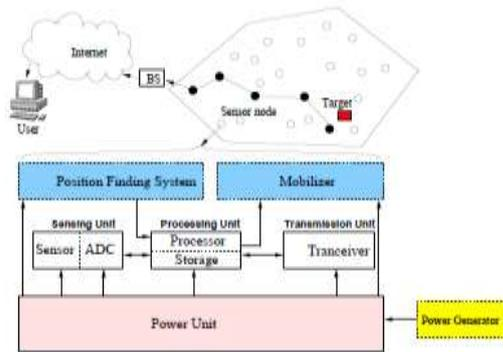
Fig 1: Components of Sensor node components
