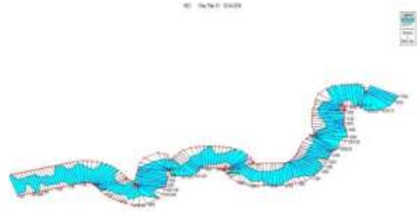
Fig 3: River boundary with the xs cut section in HEC-RAS after processing the data
