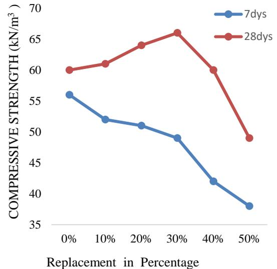
**Figure 3.1:** Compressive Strength Of 7 & 28 Days
