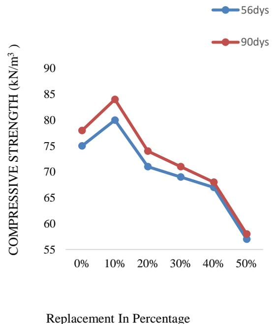
**Figure 3.2:** compressive strength of 56&90 days
