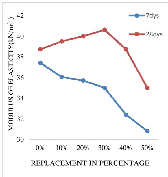
Figure 3: Static Modulus of Elasticity
