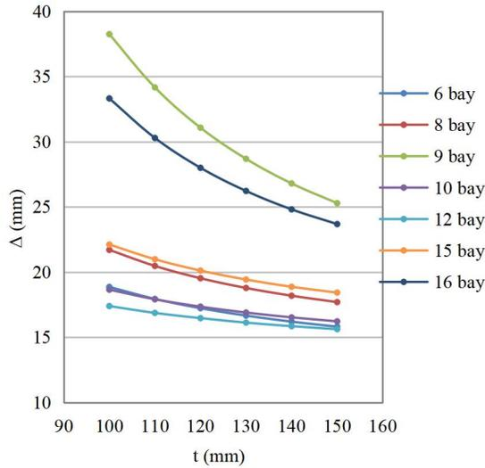
Fig. 4: Variation of displacement ( $\Delta$ ) with thickness ( $t$ ) for  $H = 1.0$  m in V type of FPR
