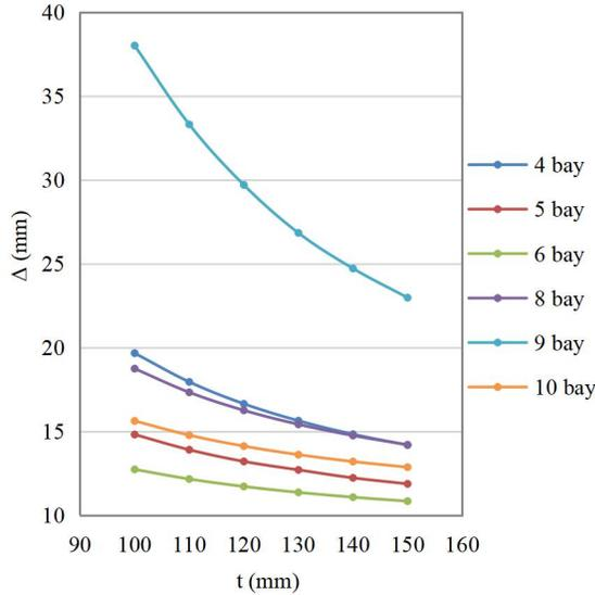
Fig.7: Variation of displacement ( $\Delta$ ) with thickness ( $t$ ) for  $H = 1\text{m}$  in Trapezoidal type of FPR
