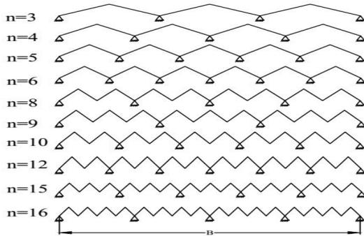
**Fig. 2:** Cross section of V-type of FPR with different number of bays; n = Number of bays; B = Total width
