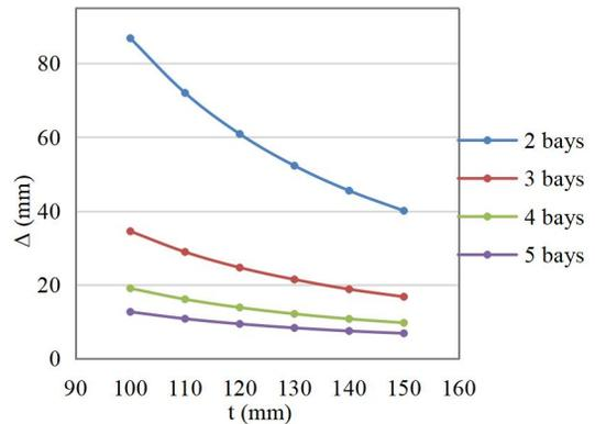
Fig.9: Variation of displacement ( $\Delta$ ) with thickness ( $t$ ) for  $H = 2\text{ m}$  in Trapezoidal type of FPR
