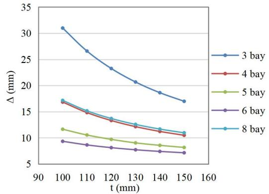
Fig.8: Variation of displacement ( $\Delta$ ) with thickness ( $t$ ) for  $H = 1.34\text{ m}$  in Trapezoidal type of FPR
