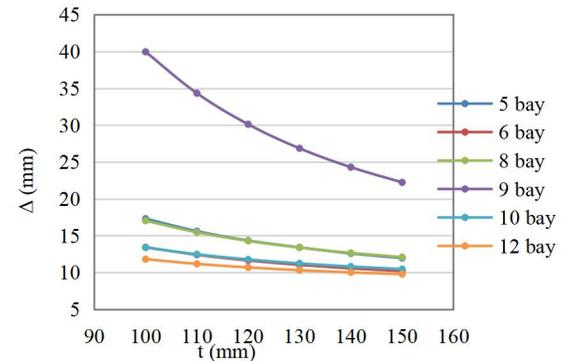
Fig. 5: Variation of displacement ( $\Delta$ ) with thickness ( $t$ ) for  $H = 1.34$  m in V type of FPR
