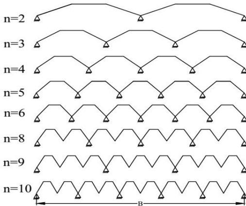
**Fig.3:** Cross section of Trapezoidal type of FPR with different number of bays; n = Number of bays; B = Total width
