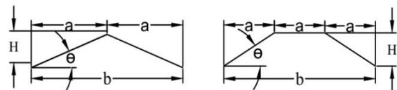
**Fig 1:** Typical cross section of (i) V type of FPR; (ii) Trapezoidal type of FPR;
