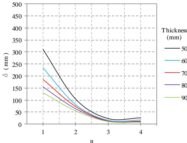
**Fig.5:** Displacement ( $\delta$ ) for cylindrical shell of height 2.5 m
