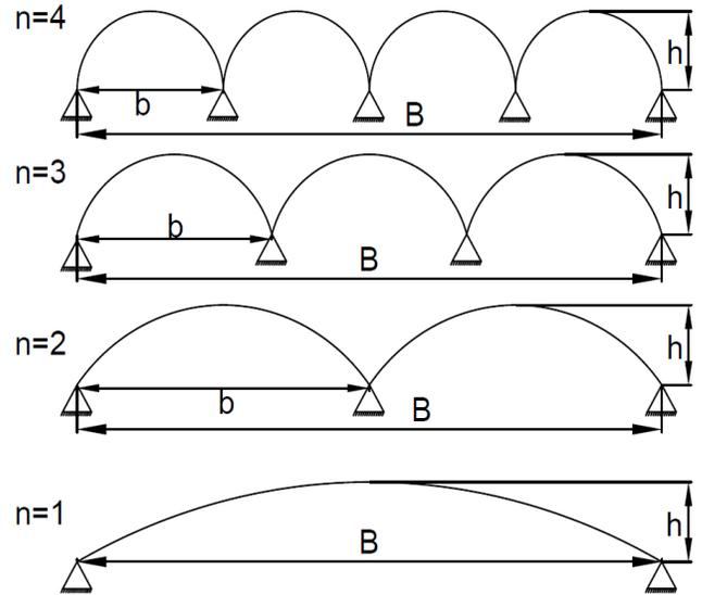
**Fig.3:** Cross section of cylindrical shell roof with different number of bays. n = Number of bays; h = Height; b = bay width; B = Total width of plan
