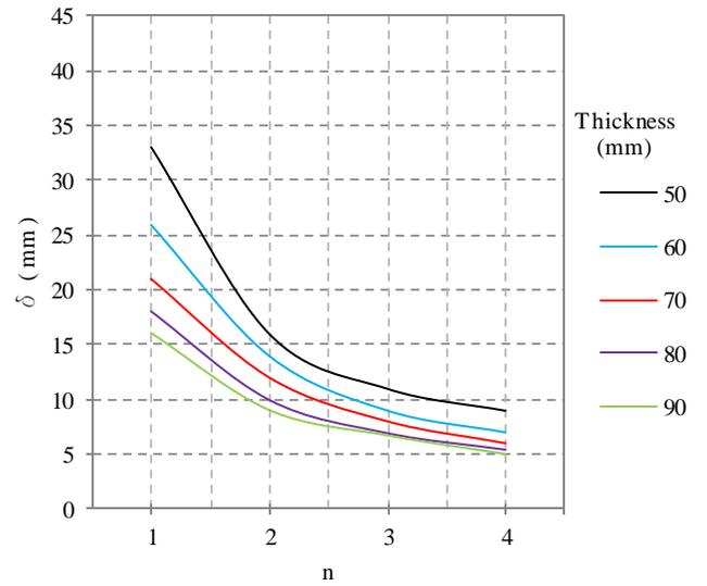
Fig.11: Displacement ( $\delta$ ) for hyperbolic paraboloid shell of height 2.22 m
