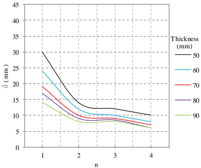
Fig.10: Displacement ( $\delta$ ) for hyperbolic paraboloid shell of height 2.5 m
