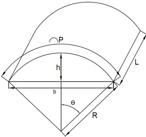
**Fig.1:** Isometric view of cylindrical shell roof (CS). h = Height; R = Radius;  $\theta$  = Semi-central angle; L = Length; b = bay width; P = Circumference
