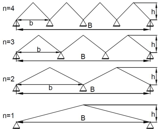
**Fig.4:** Cross section of Hyperbolic Paraboloid shell roof with different number of bays. n = Number of bays; h = Height; b = bay width; B = Total width of plan
