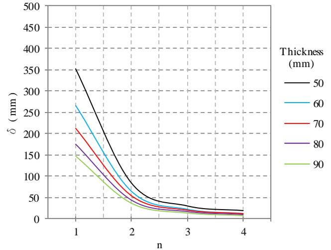
**Fig.6:** Displacement ( $\delta$ ) for cylindrical shell of height 2.22 m
