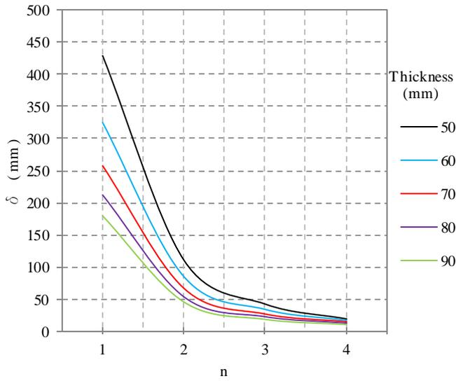
Fig.8: Displacement ( $\delta$ ) for cylindrical shell of height 1.818 m
