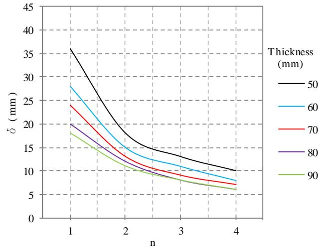
Fig.12: Displacement ( $\delta$ ) for hyperbolic paraboloid shell of height 2 m
