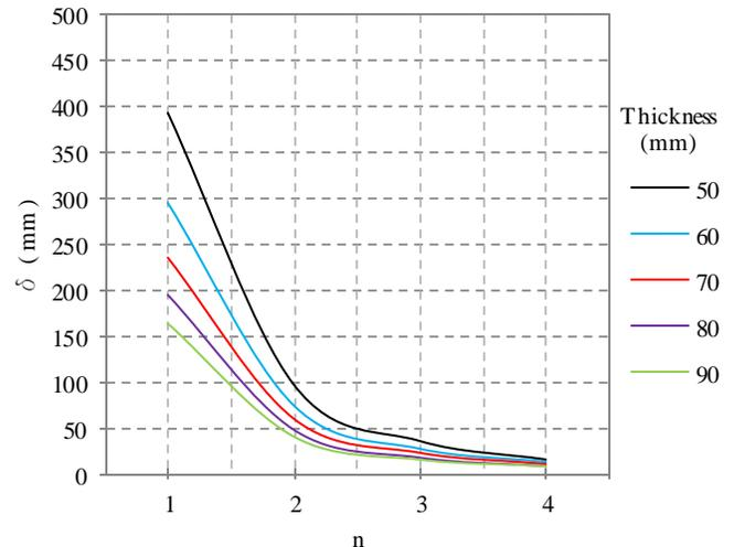
**Fig.7:** Displacement ( $\delta$ ) for cylindrical shell of height 2 m
