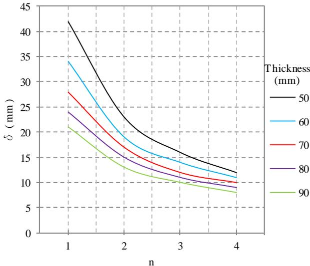
**Fig.14:** Displacement ( $\delta$ ) for hyperbolic paraboloid shell of height 1.67 m
