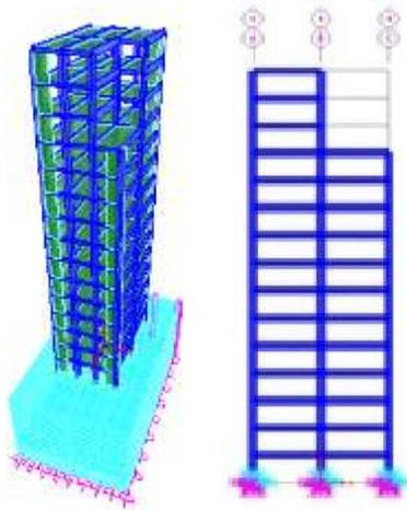
Fig.4: Continuum model with Vertical Irregularity
