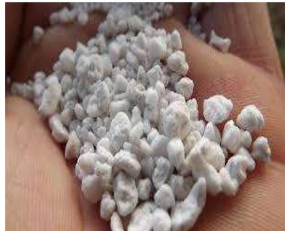
**Fig. 1:** Expanded perlite aggregate
