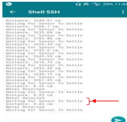
Fig.10: Ultrasonic sensor reading on mobile for landmine
