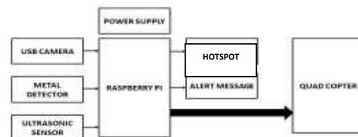
Fig. 1: Flow Chart of aerial landmine detection
