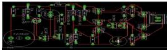
Fig. 4: PCB board design of sensor
