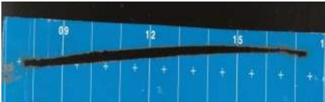
**Figure 4:** Data Cards showing maximum sunshine duration hours which is the burnt card length
