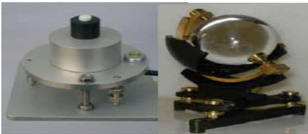
**Figure 3:** Pyranometer KDS-051 & Sunshine recorder for measurement of solar radiation and sunshine hours
