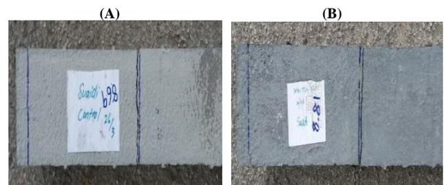
Fig. 9: Crack Pattern of LFC-BSP-POFA without CFRP Strengthening with (A) (0% BSP 0% POFA), and (B) (1% BSP 0% POFA).
