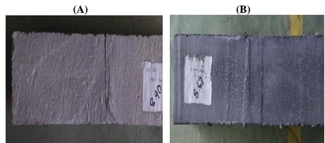
Fig. 10: Crack Pattern of LFC-BSP-POFA without CFRP Strengthening with (A) (0% BSP 15% POFA), and (B) (1% BSP 15% POFA).
