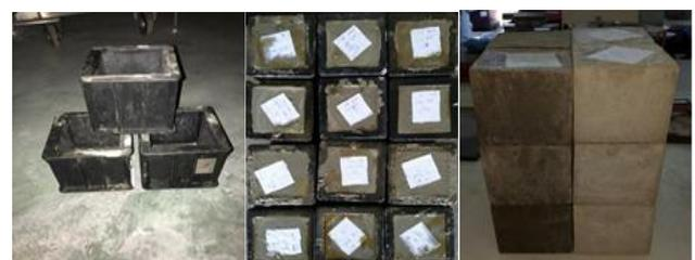
Fig. 3: Cubes Mould (Left), Wet Mix LFC-BSP-POFA in the Mould (Center), the LFC-BSP-POFA Once Demoulded (Right).
