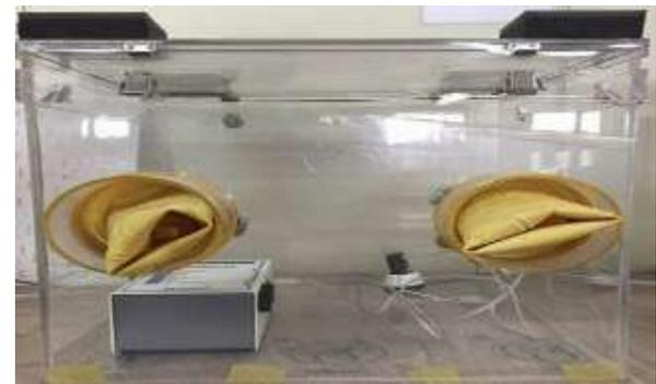
**Figure 3:** Chamber test conditions for radon adsorption
