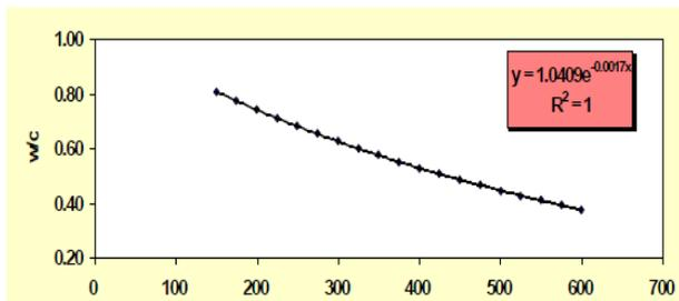
Fig. 8: Correlation W/C to Compressive Strength.
