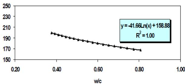
Fig. 7: Free Water Requirement per M3 to Slump 12 Cm.
