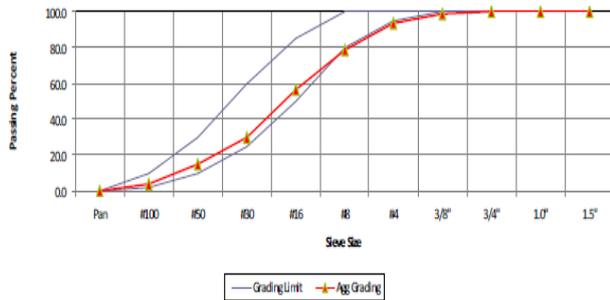
Fig. 5: Grading combined of Bangka sand and M-Sand.
