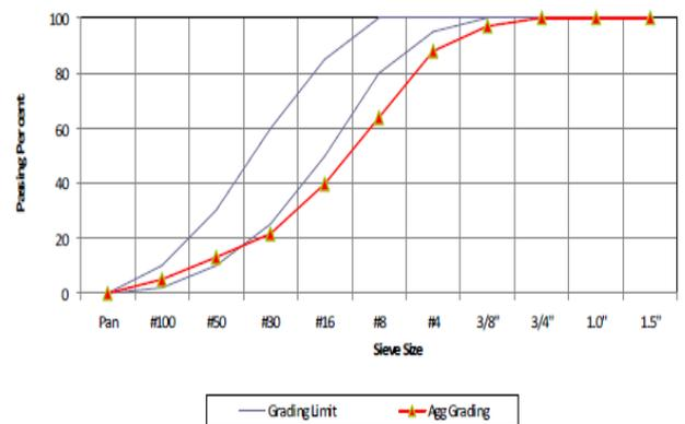
**Fig. 4:** Grading Material of M-Sand.
