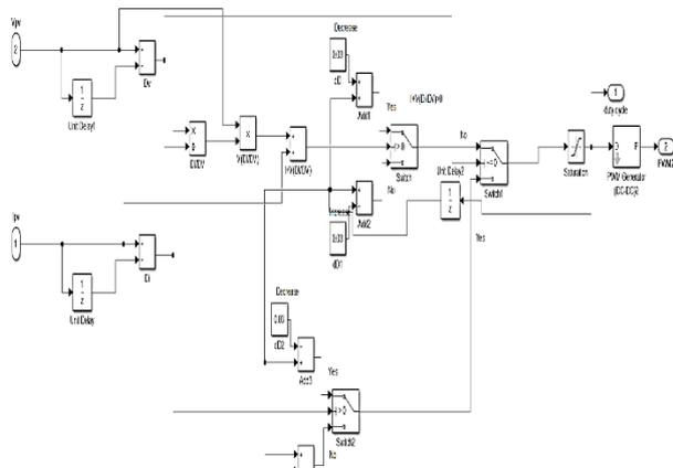
**Fig. 4.5:** Simulation of Incremental Conductance Method Algorithm.
