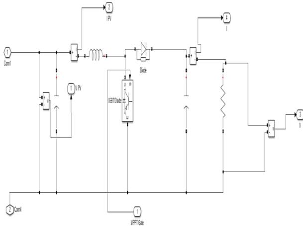
**Fig. 4.3:** Simulation of Boost Converter for the Output Voltage as 600 V DC.
