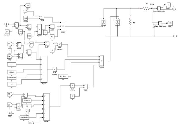
Fig. 4.1: Simulation of Single PV Cell.
