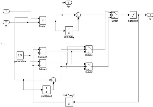
**Fig. 4.4:** Simulation of Perturb & Observe MPPT Method Algorithm.
