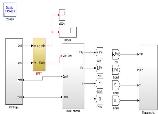
Fig. 4.2: Complete Setup of PV System with Boost Converter and MPPT Controller.
