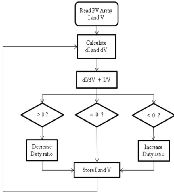
Fig. 3.2: Basic Algorithm for Incremental Conductance Method.
