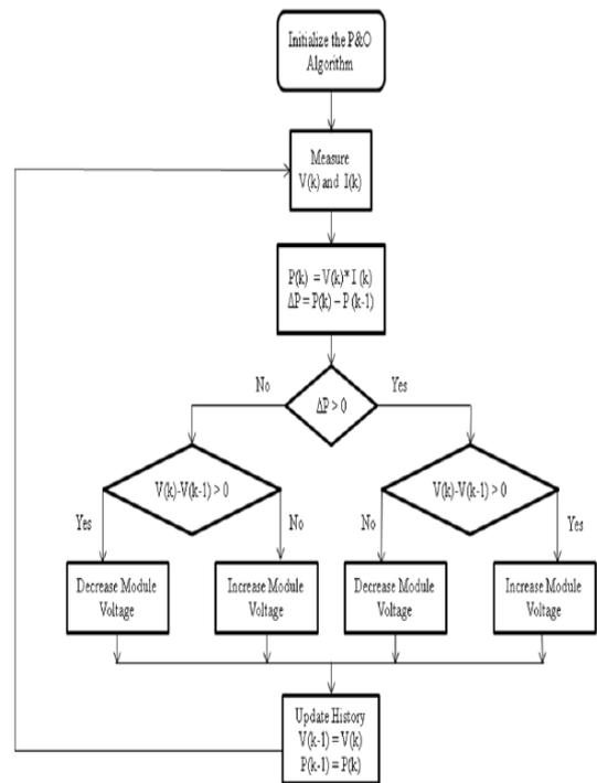
Fig. 3.1: Algorithm for Perturb and Observe Method.
