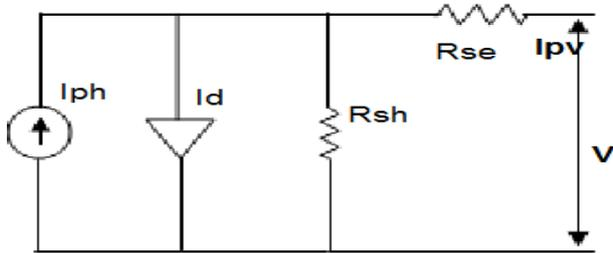
Fig. 2.1: Equivalent Circuit of PV Cell.
