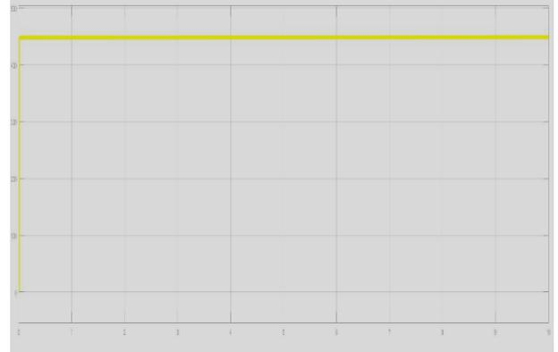
**Fig. 4.6: A)** Voltage Profile of the Boost Converter with P&O Method.
