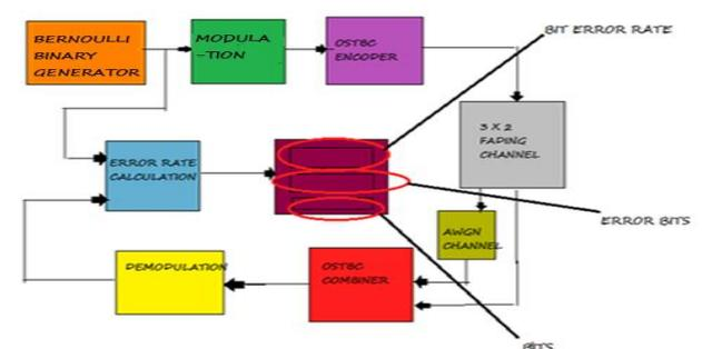
Fig. 7: Designing Block Diagram for Multiple Input and Multiple Output.
