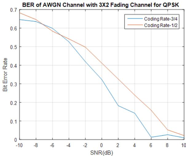
Fig. 19: BER vs SNR for QPSK.
