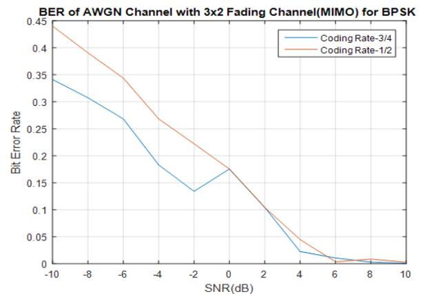
Fig. 16: BER Vs SNR for BPSK Technique Fig. 16 Gives Variation of BER for Various Values of SNR for 3/4 and 1/2 Coding Rate.
