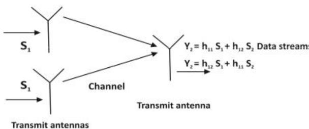
Fig. 3: Multiple Input-Single Output Assume [2] Transmitting Antennas and [1] Receive Antenna. There Will Be One Received Signal.
