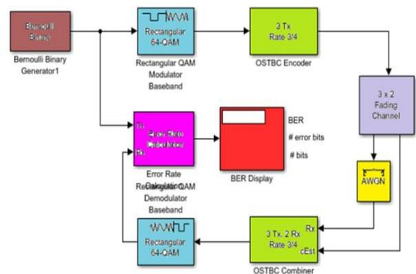
Fig. 21: 64 QAM with MIMO (3/4 Coding Rate).
