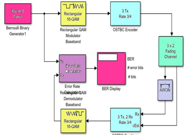
Fig. 20: 16 QAM with MIMO (3/4 Coding Rate)
