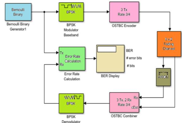
Fig. 15: BPSK with MIMO (3/4 Coding Rate).
