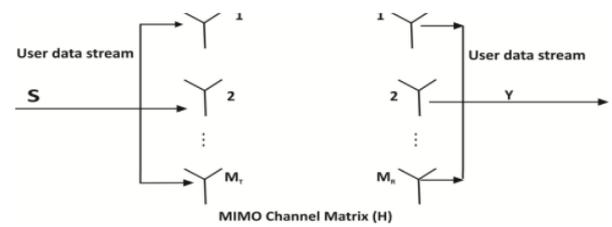
Fig. 4: MIMO Antenna Configuration.
