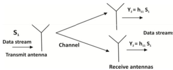
Fig. 2: Single Input Multiple Output.
