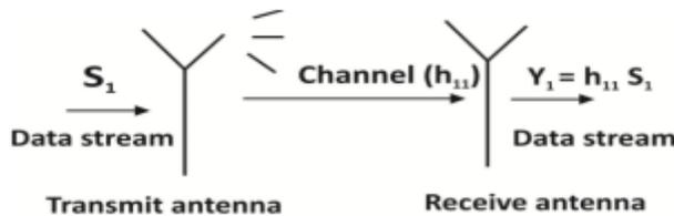
Fig. 1: Single Input-Single Output (SISO) when the Signal is Propagating through an Environment, the Signal Undergoes Fading. the Single Input Single Output (SISO) is Illustrated in Fig.1.
