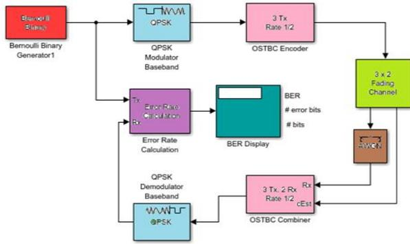
Fig. 18: QPSK with MIMO (1/2 Coding Rate).
