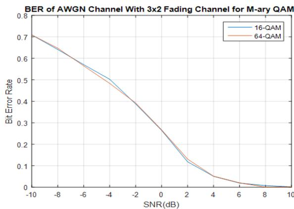
Fig. 22: BER vs. SNR for 16-QAM and 64-QAM (III) Channel Capacity.
