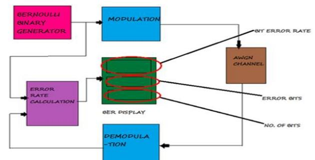
Fig. 6: Simulink Block Diagram for Single Input and Single Output.
