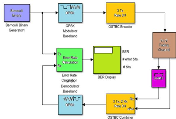
Fig. 17: QPSK with MIMO (3/4 Coding Rate).
