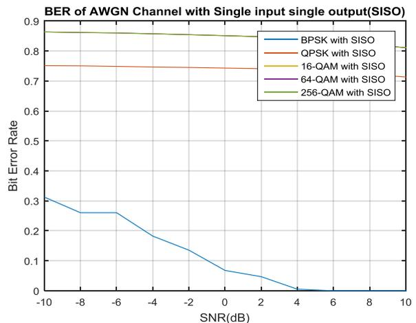
**Fig. 13:** BER of AWGN Channel with SISO by Using BPSK, QPSK, 16, 64,256-QAM
