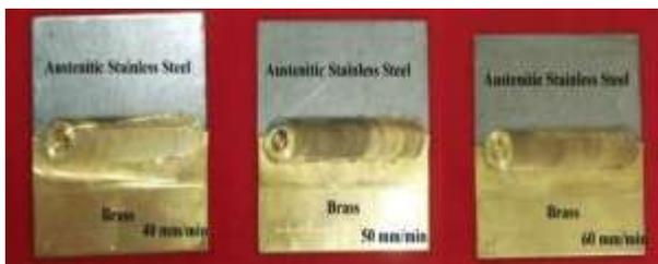
Fig 1: Friction Stir Welded Plates.
