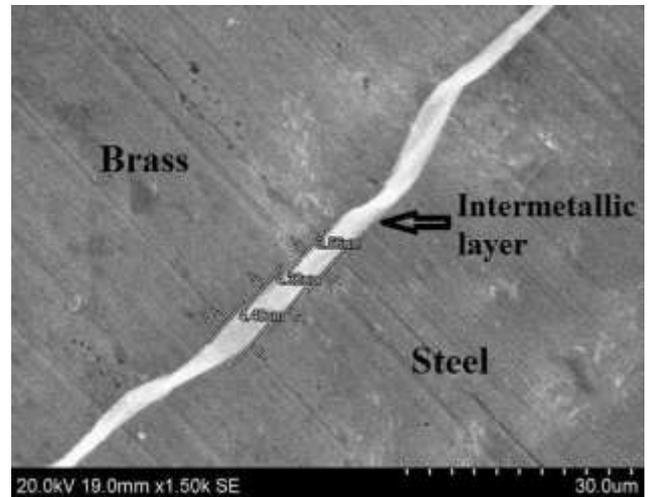
Fig 3: Intermetallic layer in interface at 550 rpm and 40 mm/min.
