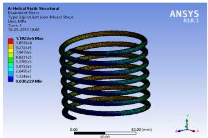
**Fig.3:** Equivalent Stress of Helical Spring
