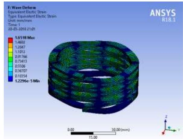
Fig.6: Equivalent (von-Mises) strain of wave spring
