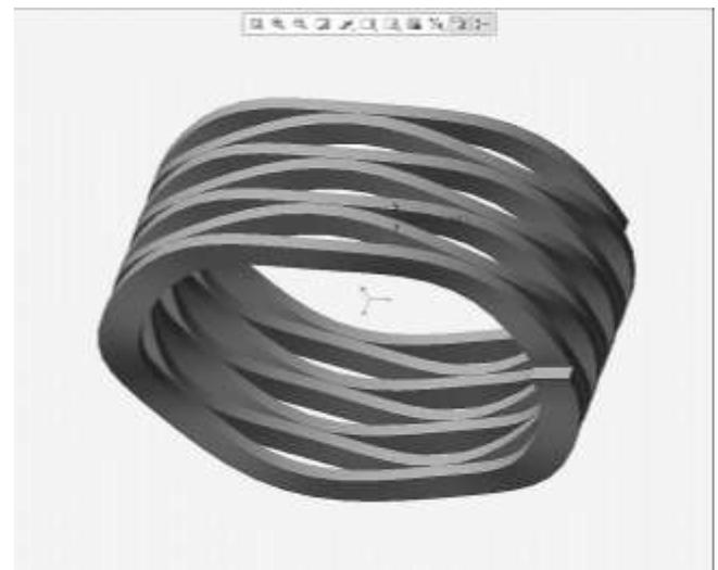
**Fig.2:** CADD Model of wave spring in CREO
