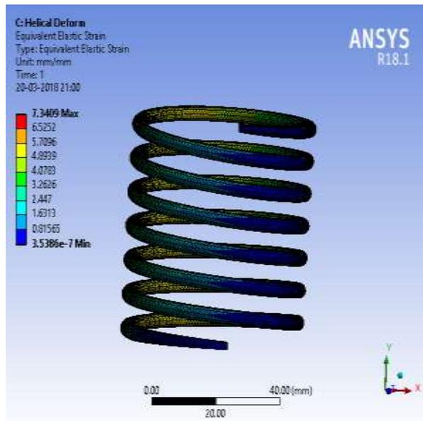
Fig.5: Equivalent (von-Mises) strain of helical spring
