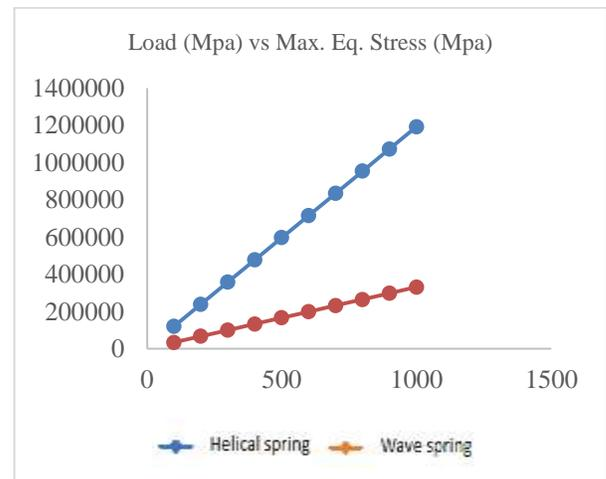
Fig.7: Comparison of load and equivalent maximum stress
