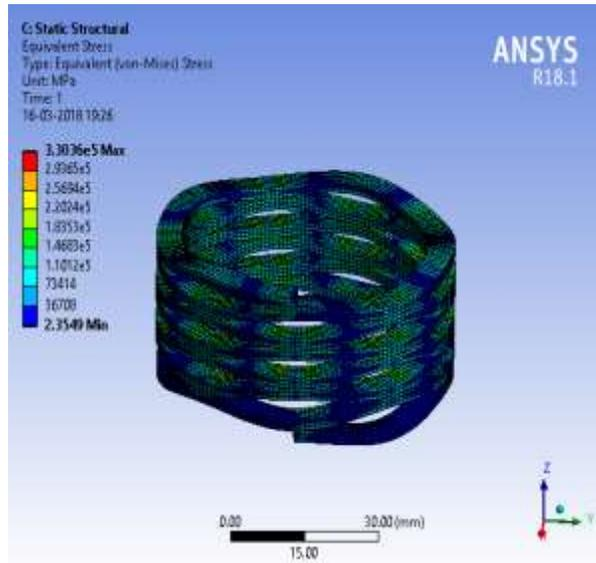
Fig.4: Equivalent stress of wave spring
