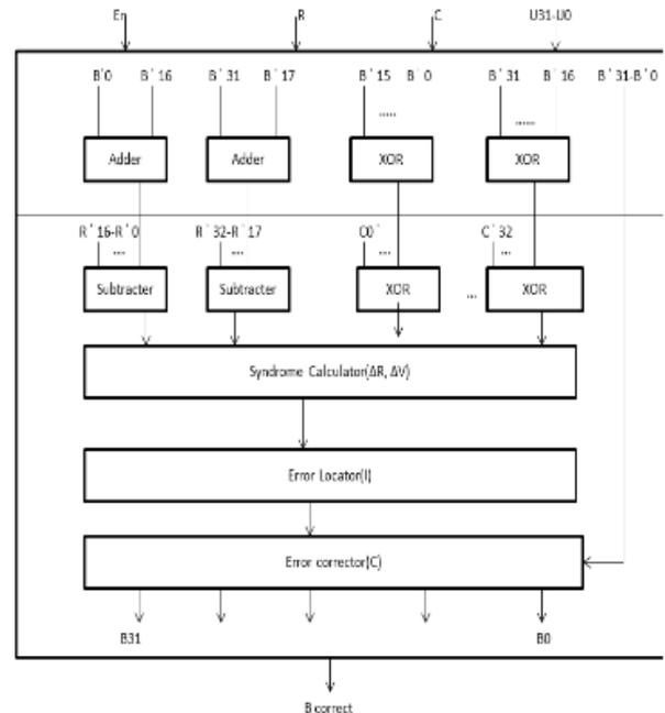
Fig. 3.7: Block Diagram of Decoder.
