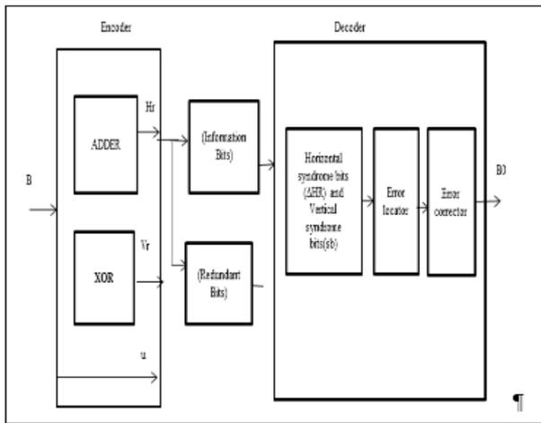
Fig. 3.1: Fault Tolerant Memory Block.
