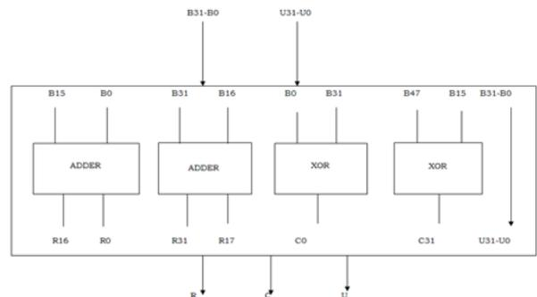
Fig. 3.4: Block Diagram of Encoder.
