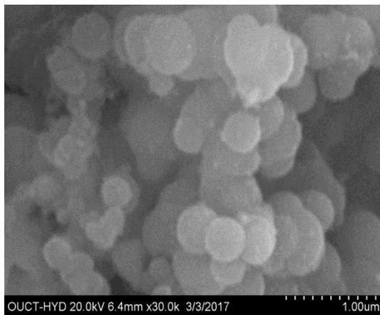
Fig. 1: SEM Image of Silica Particles.
