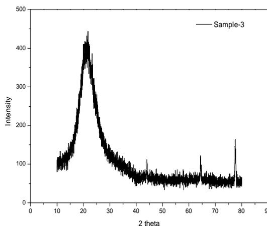
Fig. 2: XRD Characterization of Silica Particles.
