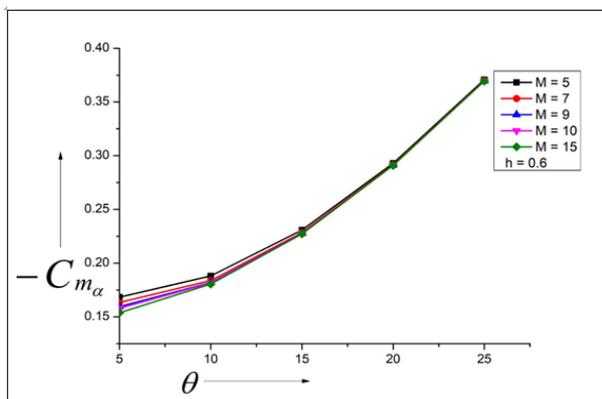
Fig. 5: Variation of Stiffness Derivative with Semi-Vertex Angle ( $\theta$ ) for  $H = 0.6$ .
