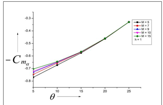
Fig. 7: Variation of Stiffness Derivative with Semi-Vertex Angle ( $\theta$ ) for  $H = 1.0$ .
