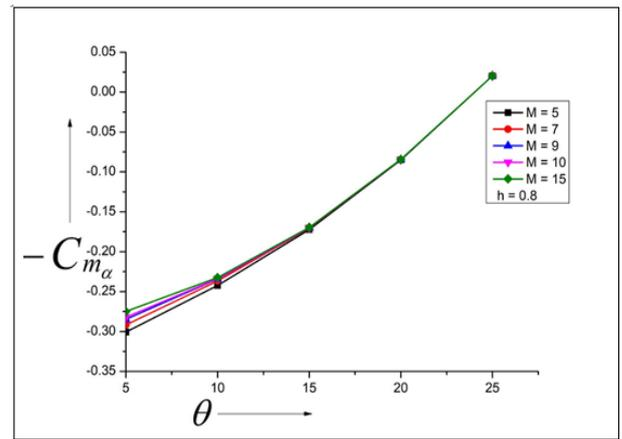
Fig. 6: Variation of Stiffness Derivative with Semi-Vertex Angle ( $\theta$ ) for  $H = 0.8$ .
