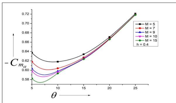
Fig. 4: Variation of Stiffness Derivative with Semi-Vertex Angle ( $\theta$ ) for  $H = 0.4$ .
