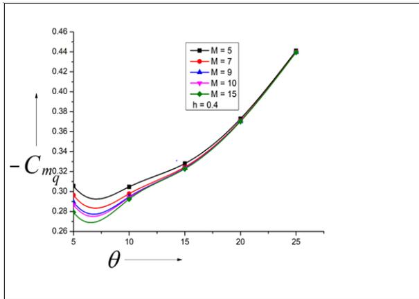
Fig. 10: Variation of Damping Derivative with Semi-Vertex Angle ( $\Theta$ ) for  $H = 0.4$ .
