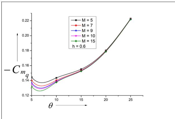
Fig. 11: Variation of Damping Derivative with Semi-Vertex Angle ( $\Theta$ ) for  $H = 0.6$ .
