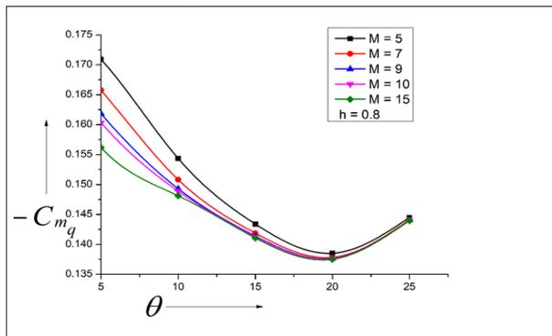
Fig. 12: Variation of Damping Derivative with Semi-Vertex Angle ( $\Theta$ ) for  $H = 0.8$ .
