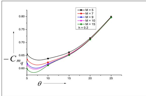
Fig. 9: Variation of Damping Derivative with Semi-Vertex Angle ( $\Theta$ ) for  $H = 0.2$ .
