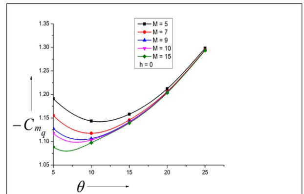
Fig. 8: Variation of Damping Derivative with Semi-Vertex Angle ( $\theta$ ) for  $H = 0.0$ .
