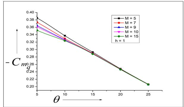
Fig. 13: Variation of Damping Derivative with Semi-Vertex Angle ( $\Theta$ ) for  $H = 1.0$ .
