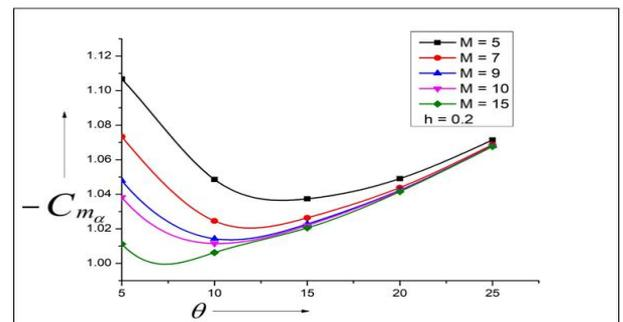
Fig. 3: Variation of Stiffness Derivative with Semi-Vertex Angle ( $\Theta$ ) for  $H = 0.2$ .
