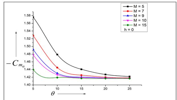
Fig. 2: Variation of Stiffness Derivative with Semi-Vertex Angle ( $\Theta$ ) for  $H = 0.0$ .
