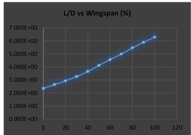
Fig. 8.6: L/D ratio vs Wingspan Graph.
