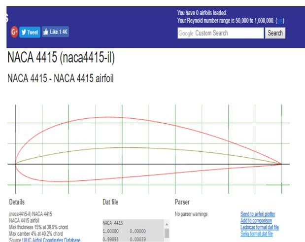
Fig. 3.2: Airfoil Tools (NACA 4415).
