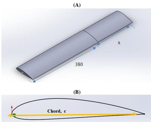
Fig. 3.4: Half Wing Dimension of NACA 4415 (AoA = 1°).
