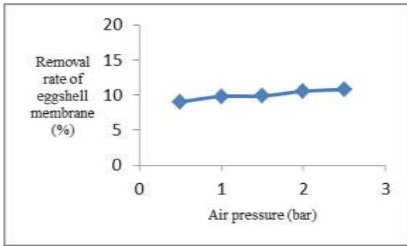
Fig. 2: Effect of air pressure on duck eggshell membrane removal.
