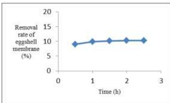
Fig. 4: Effect of residence time on duck eggshell membrane removal.
