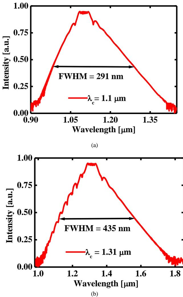
Figure 3: (a) SC spectrum at center wavelengths 1.1  $\mu\text{m}$  and (b) SC spectrum at center wavelengths 1.31  $\mu\text{m}$ .
