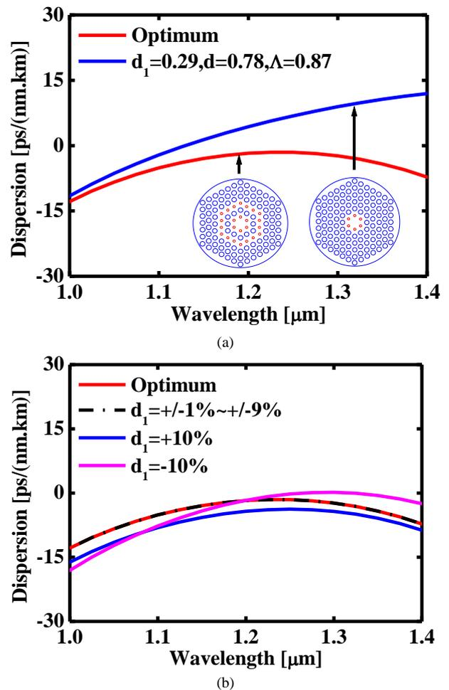
Figure 4: (a) Effect of third ring air hole diameter  $d_1$  on the dispersion behavior with  $d_1 = 0.29 \mu\text{m}$ ,  $d = 0.78 \mu\text{m}$ , and  $\Lambda = 0.87 \mu\text{m}$ , and (b) Chromatic dispersion variation after changing small air hole diameter  $d_1$ .
