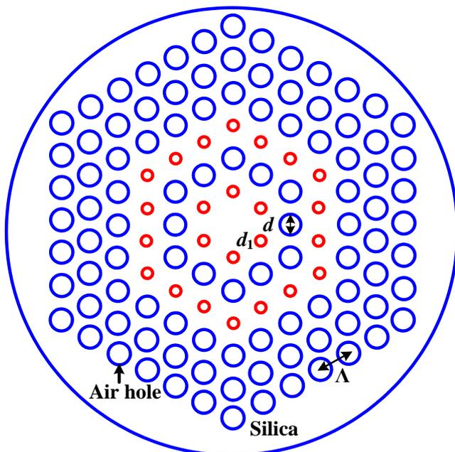
Figure 1: Architecture of the proposed six-ring highly nonlinear PCF.
