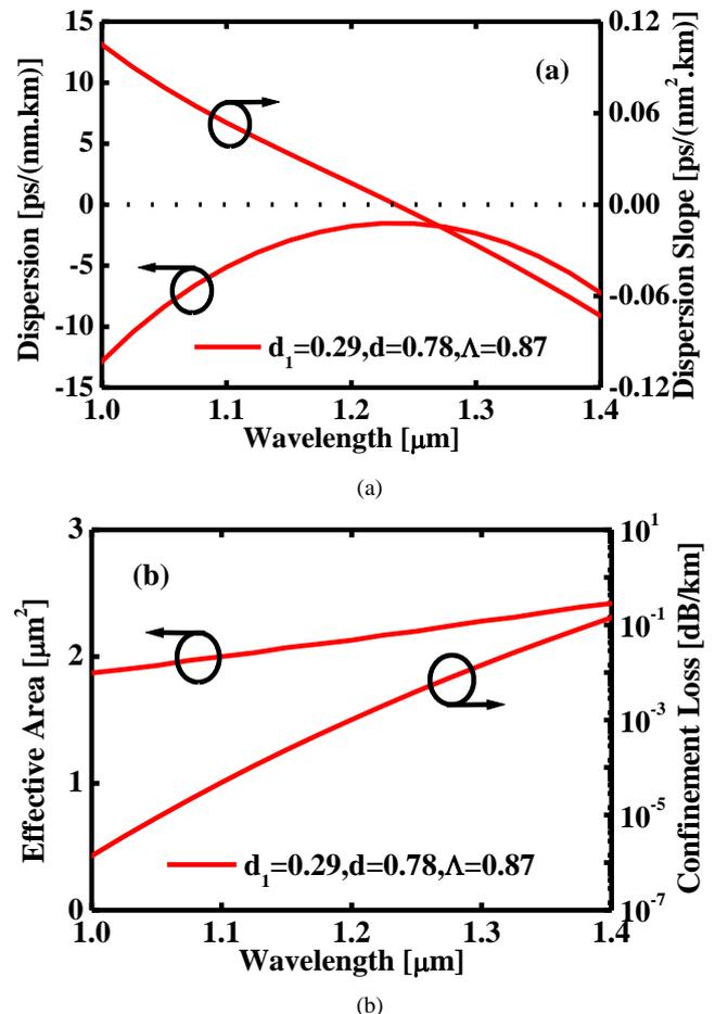
Figure 2: (a) Dispersion property and property of dispersion slope and (b) Property of effective area and property of confinement loss.
