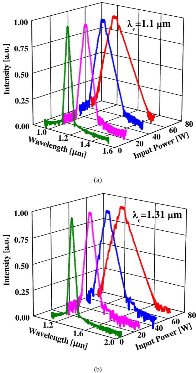
**Figure 5:** Optical intensity at center wavelengths (a) 1.1  $\mu\text{m}$  and (b) 1.31  $\mu\text{m}$  of the proposed HN-PCF in different input powers.
