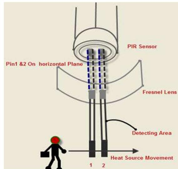
Fig 1.2: Construction of PIR sensor
