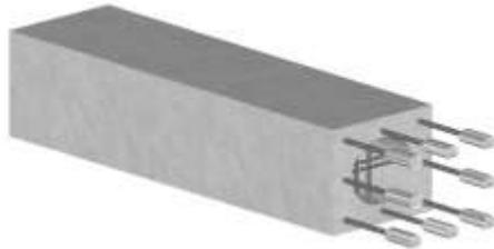
Figure 2: Hollow-PC Column
