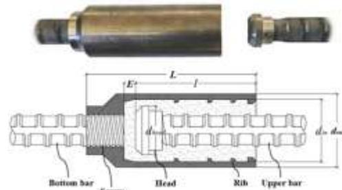
Figure 3: Head-Splice Sleeve
