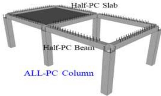
Figure 1: Half-slab method
