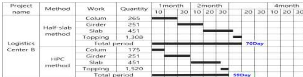
Figure 5: Construction period analysis of case B
