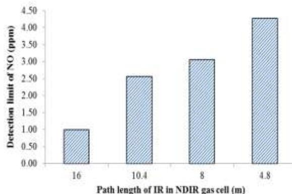
Figure 5: Relationship between detection limit of NO and optical path length of the gas cell.
