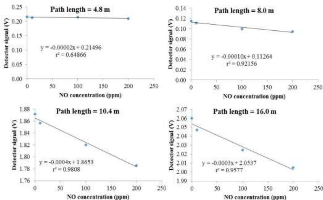
Figure 4: Variations of detector signals associated with NO concentrations and optical path lengths.
