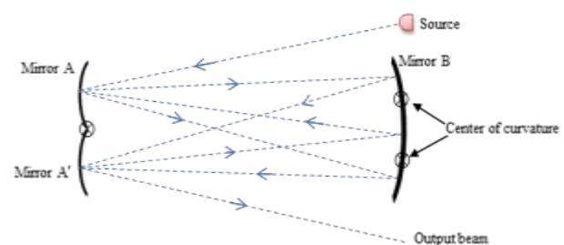
Figure 1: Diagram of White cell principle.
