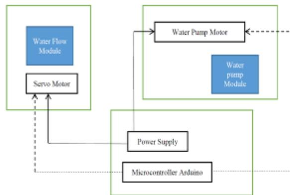
Fig. 5: block diagram of aquaponics system
