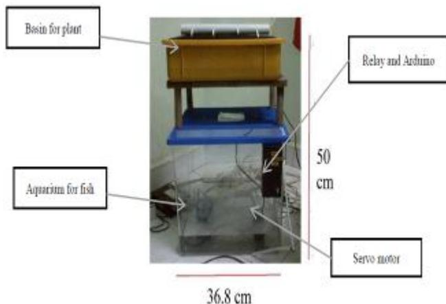
Fig. 4: Aquaponics Design with components
