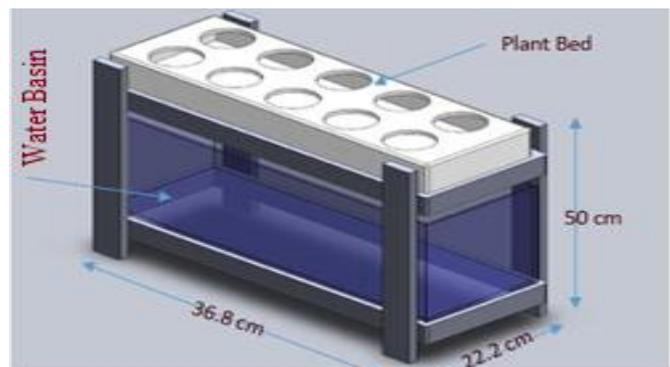
**Fig. 2:** Our Aquaponics Design using Solidworks.
