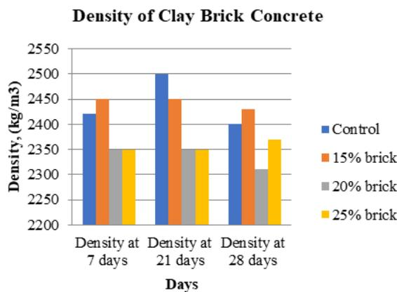
Fig 3: Density of hardened clay brick concrete
