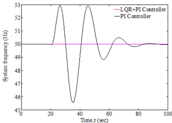
Fig. 7: The frequency changes for the power system
