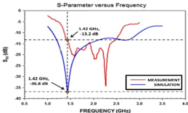
Fig. 3: S-parameter graph between simulation and measurement.
