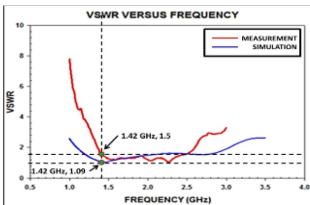
Fig. 4: VSWR plotting graph between simulation and measurement
