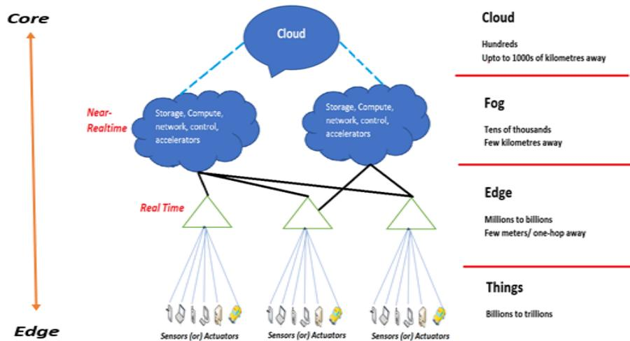
**Fig. 3:** Architecture: Edge, Fog and Cloud Computing Paradigm.
