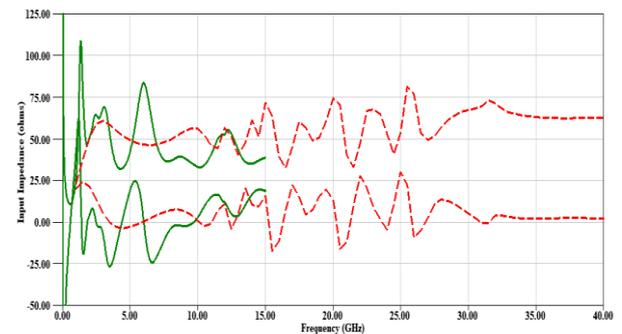
**Fig. 5:** Input Impedance Plot of the Proposed Antenna. (Solid Curve Represents Measured and Dashed Curve Represents Simulated).
