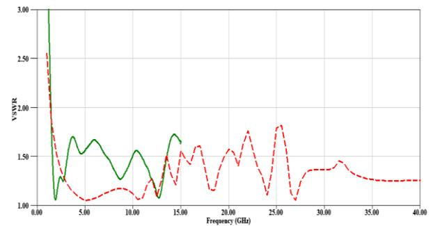
**Fig. 4:** VSWR Plot of the Proposed Antenna. (Solid Curve Represents Measured and Dashed Curve Represents Simulated).
