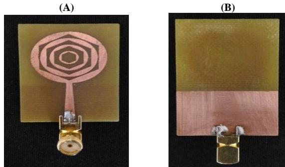
**Fig. 2:** Photograph of the Fabricated Prototype of the Proposed Antenna (A) Top View and (B) Bottom View Only Real Impedance.
