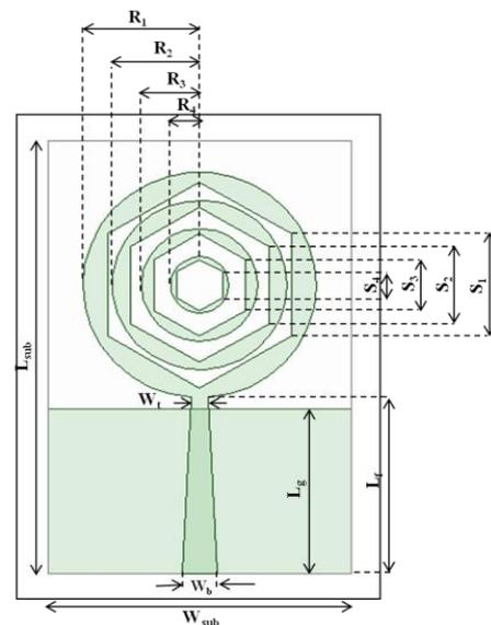
**Fig. 1:** Geometrical Structure of the Proposed Antenna.  $L_{sub}$  = Length of Substrate,  $W_{sub}$  = Width of Substrate,  $L_f$  = Length of Feed,  $L_g$  = Length of Ground,  $R$  = Radius of Circular Patch,  $S$  = Side Length of Hexagonal Slot,  $W_b$  = Bottom Width of Feed Line,  $W_t$  = Top Width of Feed Line.
