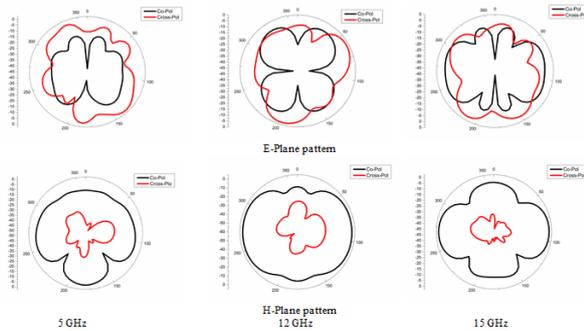
**Fig. 8:** Measured Radiation Patterns of the Proposed Antenna at Different Frequencies both in E-Plane and H-Plane.
