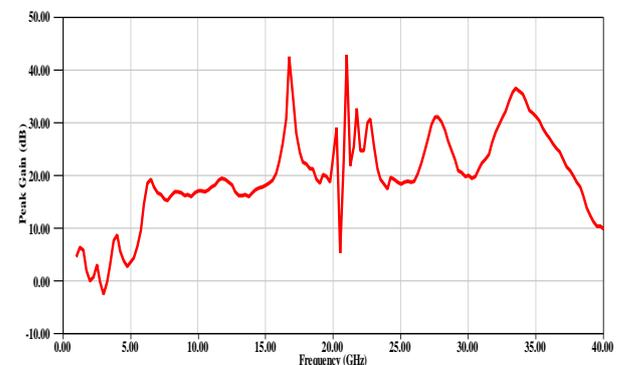
**Fig. 6:** Simulated Peak Gain versus Frequency of the Proposed Antenna.
