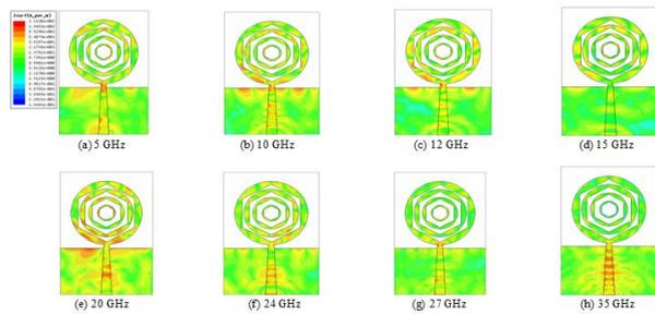
**Fig. 7:** Simulated Surface Current Density of the Proposed Antenna at Few Selected Frequencies.
