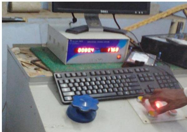
**Fig 5:** Digital Deflectometer
