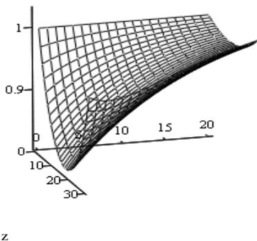
Figure 4.: Oxygen compressibility factor as a function of pressure (on the axis from 0 to 30 MPa) and temperature (on the axis from 0 to 30 in tens of Kelvin). Calculations made using the van der Waals equation.
