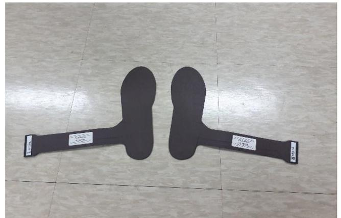
Fig.2: Insoles with built-in foot plantar pressure sensors
