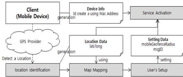
Fig. 1: Activation process of connected car service
