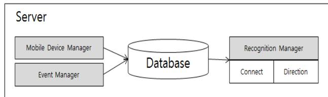
Fig 2: Architecture of the proposed server model
