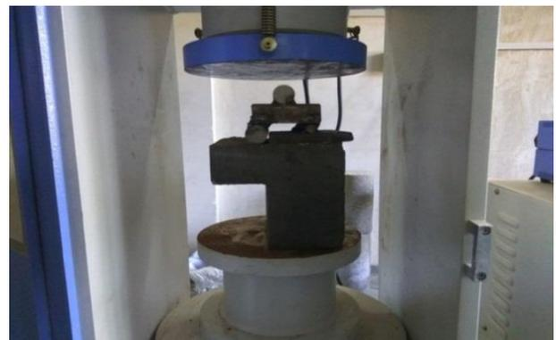
**Fig. 4:** Experimental Set Up for Shear Test.
