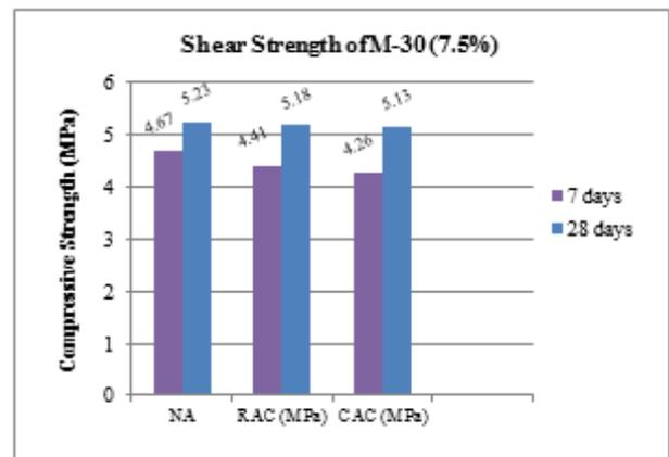
Fig. 11: Shear Strength of Selected RAC and CAC with 7.5% Met kaolin for M30.
