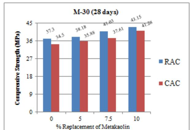
Fig. 15: At 28-Days Compressive Strength of RAC and CAC for M-30.
