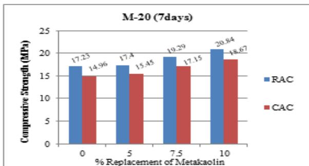
Fig. 12: At 7-Days Compressive Strength of RAC and CAC for M20.
