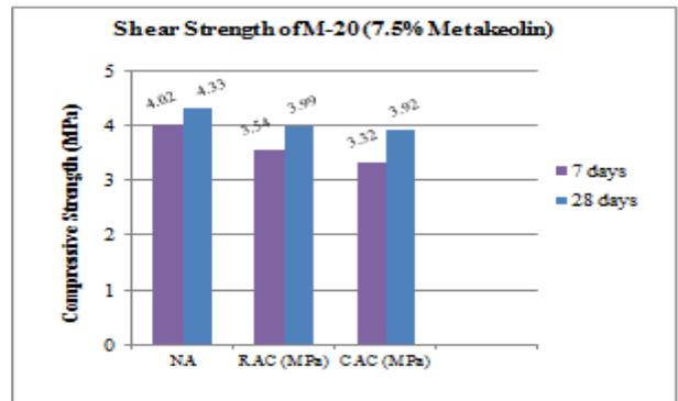
Fig. 8: Shear Strength of Selected RAC and CAC with 7.5% Metakaolin for M-20.
