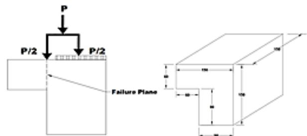
**Fig. 3:** Dimensions of Specimen and Loading Setup.
