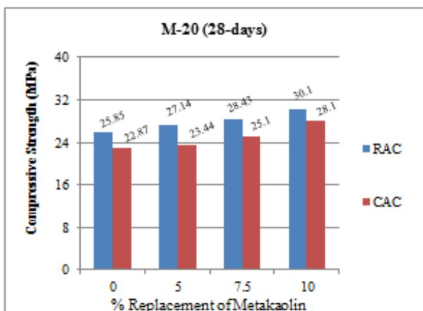
Fig. 13: At 28-Days Compressive Strength of RAC and CAC for M20.
