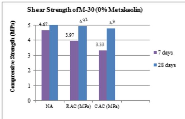
Fig. 6: At 7-Days & 28-Days, Shear Strength of Selected RAC and CAC without Metakaolin for M30.
