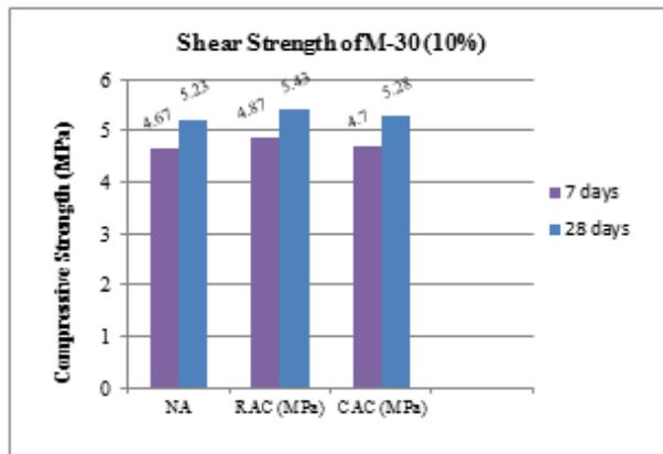
Fig. 12: Shear Strength of Selected RAC and CAC with 10% Met kaolin for M30.
