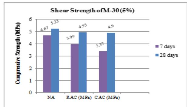
Fig. 10: Shear Strength of Selected RAC and CAC With 5% Met kaolin for M30.
