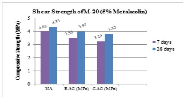
Fig. 7: Shear Strength of Selected RAC and CAC with 5% Metakaolin for M-20.
