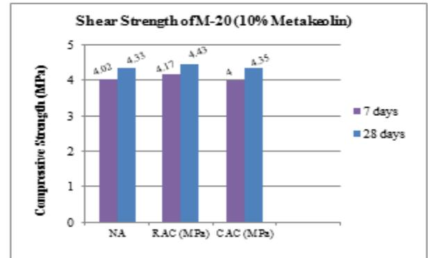
Fig. 9: Shear Strength of Selected RAC and CAC with 10% Metakaolin for M20.
