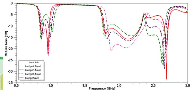
Figure 9: Parametric investigation on varying the length of the strip 'Lstrip'
