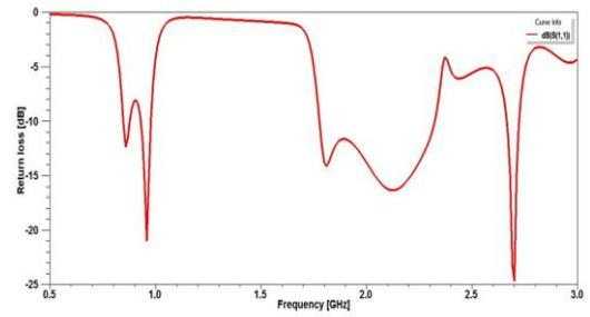
Figure 3.: Return loss plot of proposed antenna
