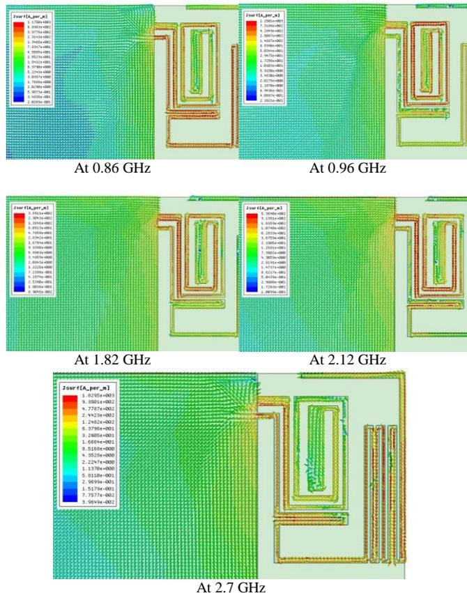
Figure 7: Surface Current Distributions at operating bands
