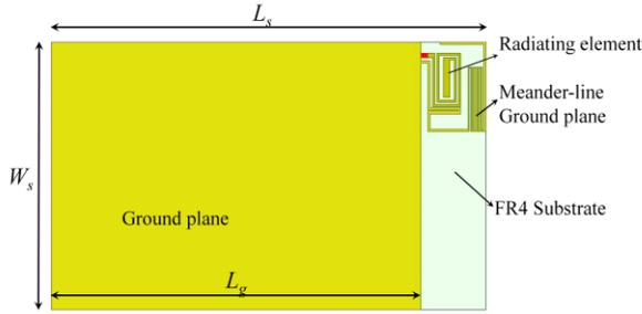
Figure 1.: Antenna Architecture
