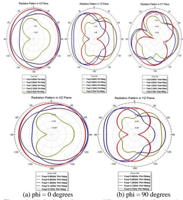
Figure 6: 2D Radiation Patterns at different operating frequencies
