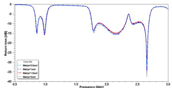
Figure 10: Parametric investigation on varying the length of the strip 'Wstrip'
